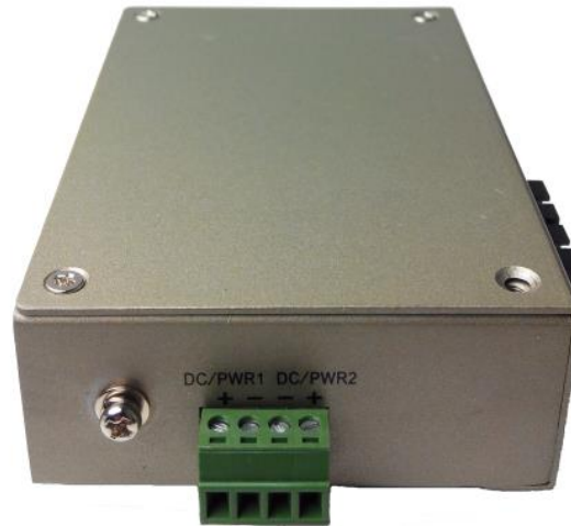
Fig. 4-5 Power Supply Terminal
