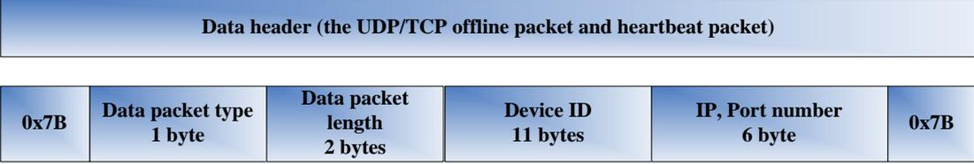
The value of the data packet type is 0x01 (heartbeat packet) or 0x82 (offline packet). The data body is empty.
