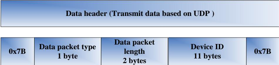
The value of the data packet type is 0x09 (terminal-reported data packet) or 0x89 (data center-delivered data packet).
