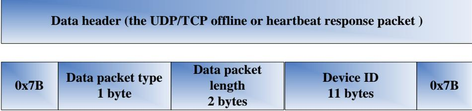
The value of the data packet type is 0x81 (heartbeat response packet) or 0x02 (offline response packet). The data header is empty. The data body is empty.
