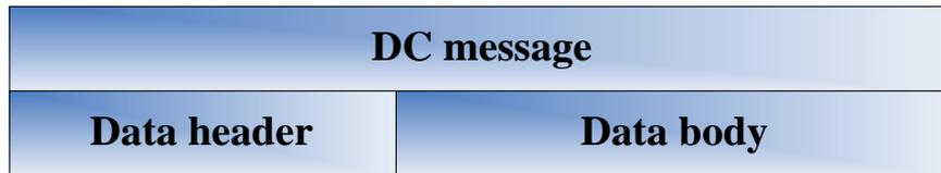
A DC message consists of two parts: data header and data body. The DC protocol defines several packet types, which are indicated by the data packet type identifier (which occupies 1 byte) in the data header. See the following table.
