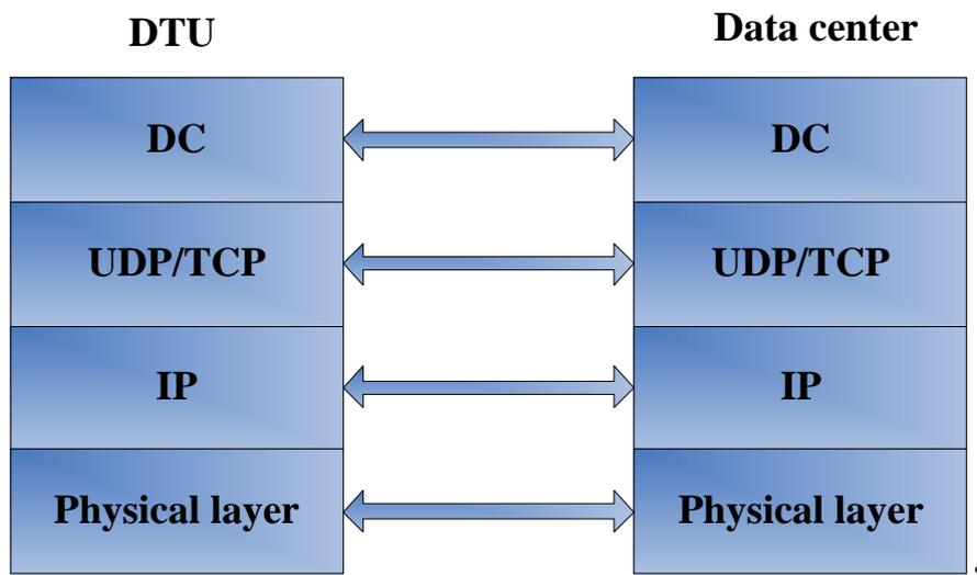
For DTU300, its physical layer is wireless cellular network, the dial link for the wireless cellular network (PPP protocol) will act as underlying bearer.
