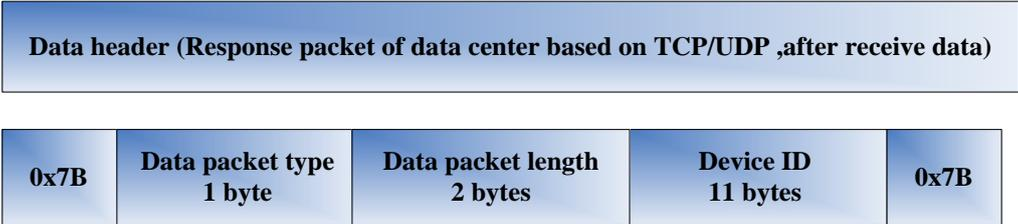
The data packet type identifier is 0x85. The data body is empty. The length of the entire data packet is 1 + 1 + 2 + 11 + 1 = 16 bytes.
