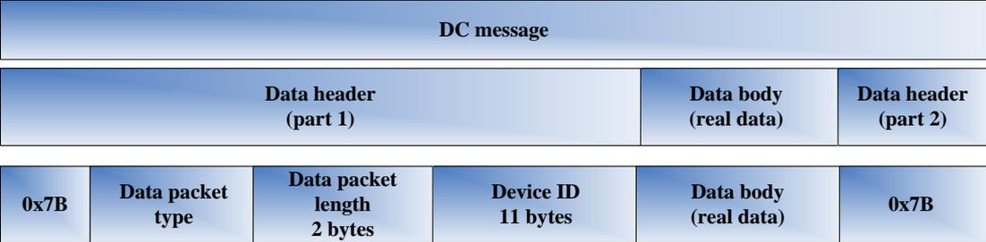
The value of the data packet type is 0x09 (terminal-reported data packet) or 0x89 (data center-delivered data packet).
