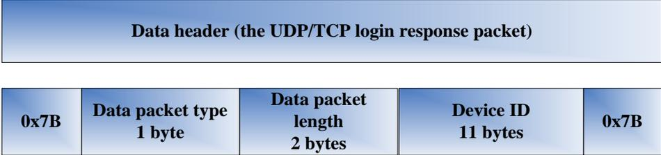
The value of the data packet type is 0x83. The data packet length is 16 bytes. The data body is empty. For example, a UDP login response packet is 7B 83 00 10 3132333400000000000000 7B.
