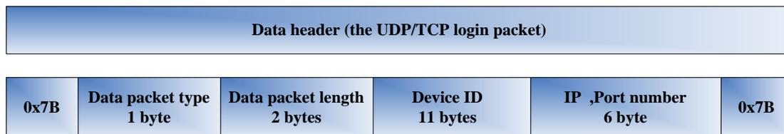
The value of the data packet type is 0x03. The IP address assigned by the wireless cellular network occupies 4 bytes. The port number occupies 2 bytes. The length of the data header is 1 + 1 + 2 + 11 + 4 + 2 + 1 = 22 bytes. Network endian is adopted. The data body is empty.
