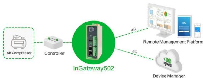
The whole system can be accessed via web and mobile app at any time from anywhere. Users can view the operation status and fault alerts of the air compressors, configure, upgrade and debug the machines remotely. This increases the operation efficiency of the equipment, shortens troubleshooting, lowers costs for maintenance as well as communication between air compressor manufacturers and customers, improving services and business performance.
