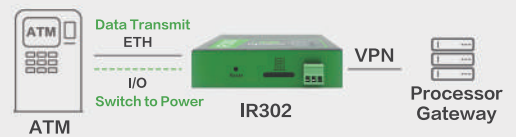
ATM Power Cycle Connected with I/O
